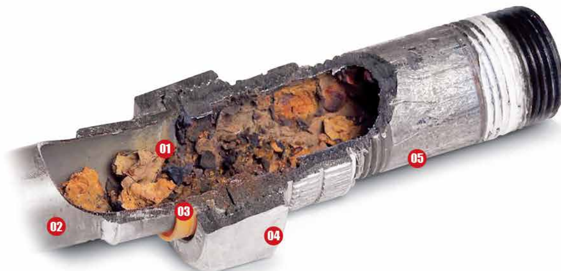
01 Corrosion | 02 Copper Pipe | 03 Plastic Liner | 04 Dielectric Union | 05 Galvanized Pipe
